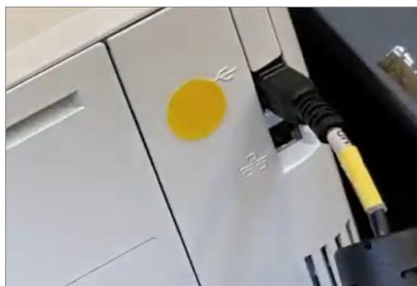
Unplug the USB cord from the back of the Printer.
