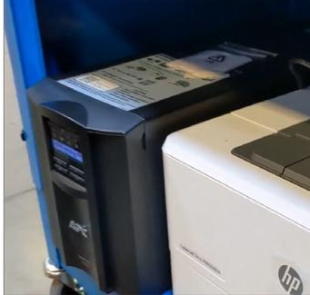
Place the UPS to the left of the printer and slide into cart.
