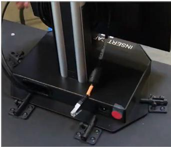
Secure the BMD tablet to the top of the cart and lock it in using the slide latches.
