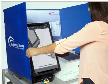
Unfold the privacy screen and position around the back of the BMD and printer. Make sure to manage all loose cords between the privacy screen and behind the BMD and printer.
