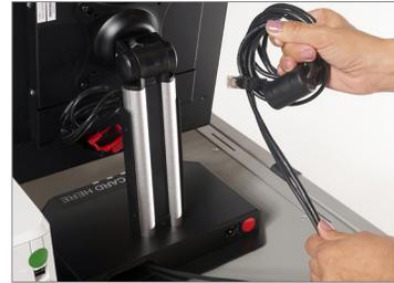
Coil the ATI cable and Printer USB cord together, then secure them behind the BMD screen (between the tablet and the stand).
