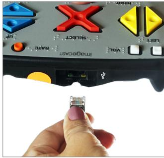
Connect the RJ-45 cable to the ATI (match orange stickers) and place ATI Unit in front of the BMD screen.
