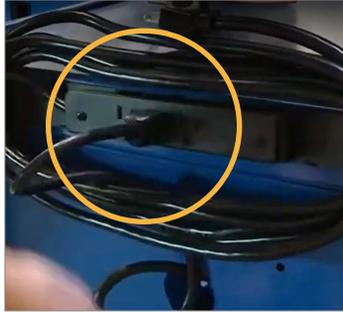
Plug the Uninterruptible Power Supply (UPS) into the power bar on the back of the cart.
