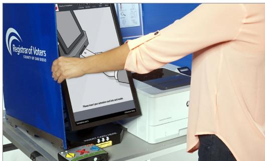
Slide the privacy screen toward the front of the booth so the teeth come out of the slots and carefully lift the screen up and over the BMD tablet, then fold closed. Set the folded screen to the side.
