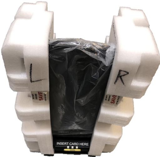
Using two hands, lift the BMD from the bag and remove foam packaging and protective plastic bag; DO NOT throw away. Place packaging and the power cord box back into the security bag for pack-out. Set the BMD on the Voting booth table.
