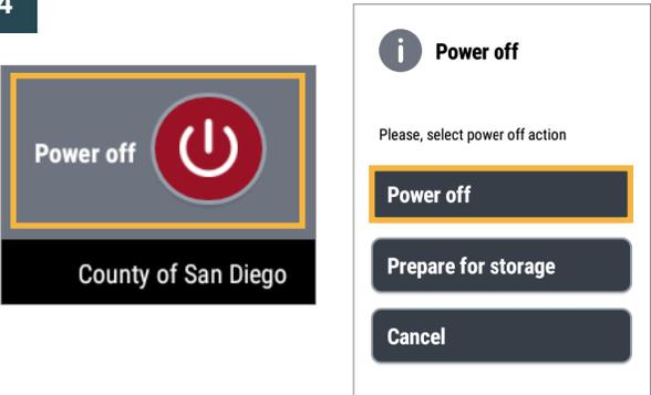
Press the Power Off button in lower right corner of the screen and when prompted, select "Power Off".
