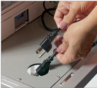
Collect both the BMD and Printer power cords and feed plug ends of cord through the left or right cord hole in the Voting Booth table.
