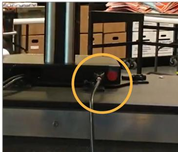
Connect the BMD power cord; then thread the power cord and the printer USB cord (from the BMD) into the hole mid-shelf.
