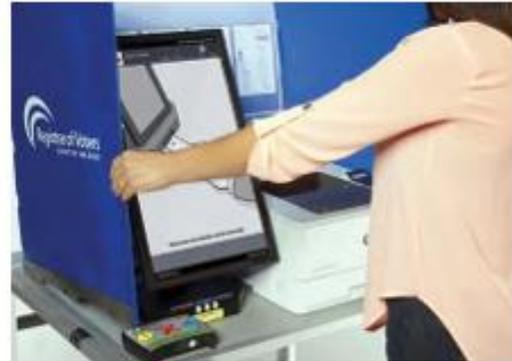
10. Open Privacy Screen and wrap around the back of the BMD and printer. Voting instruction postings should be behind the BMD and Printer and San Diego ROV logo on the outside.
