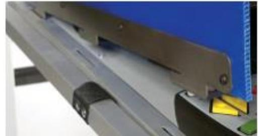
11. Insert three teeth on the left and right panels into the matching three slots in the Voting Booth table and slide back to lock in place.
