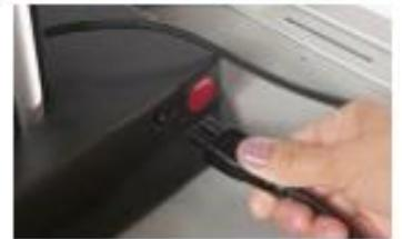
5. Plug the printer power cord into the printer (match green stickers).
