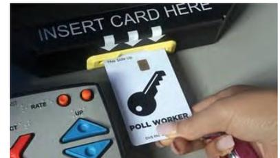
3. Insert the Poll Worker Card (found in the Official Ballot Pouch) Into the yellow slot at the bottom of the BMD with the chip facing up.
