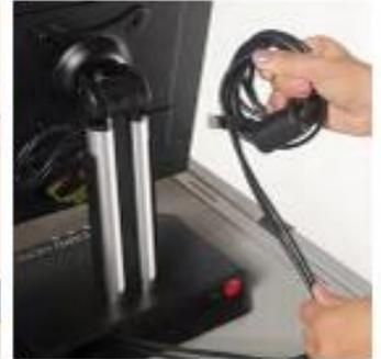
3. Locate and insert the ATI RJ-45 cable into the ATI (match orange stickers) and place ATI Unit in front of the BMD screen.
