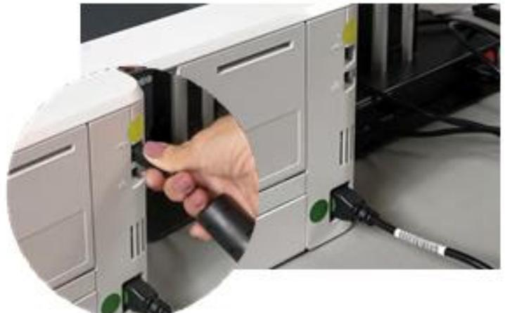
6. Insert the printer cord into the printer. This is the plug that is "D" shaped (match yellow stickers).
