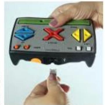
4. Locate and plug the BMD power cord into the back of the BMD (match red stickers).
